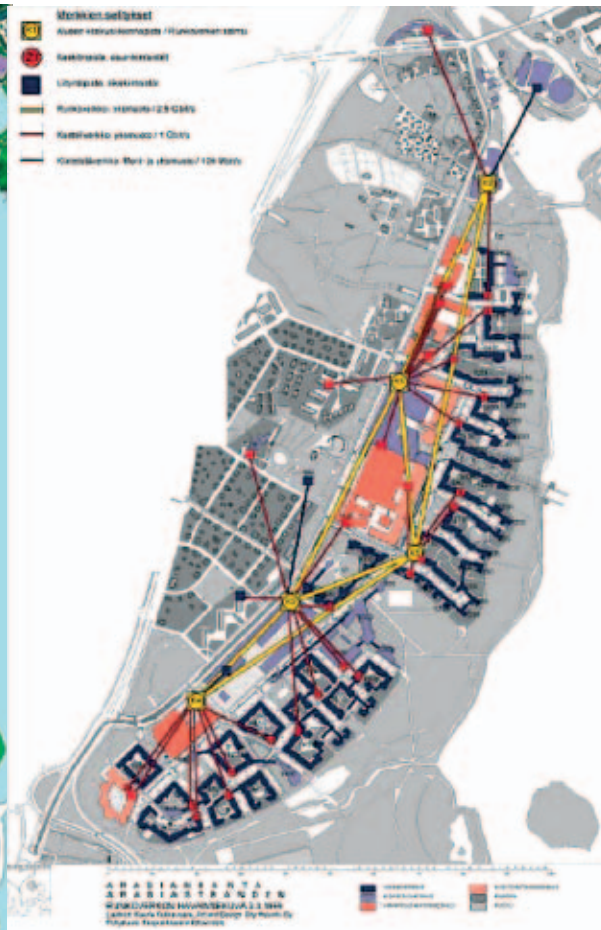
Figure 3. The 14 km net of fiber optic cables built to Arabianranta
