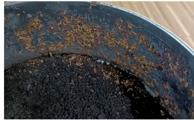
Figure 7 The metallic sample container reacted with the biochar made from soft green waste, showing corrosion (top right) and peculiar protruding crystallization on the metal bucket surface (top left)
