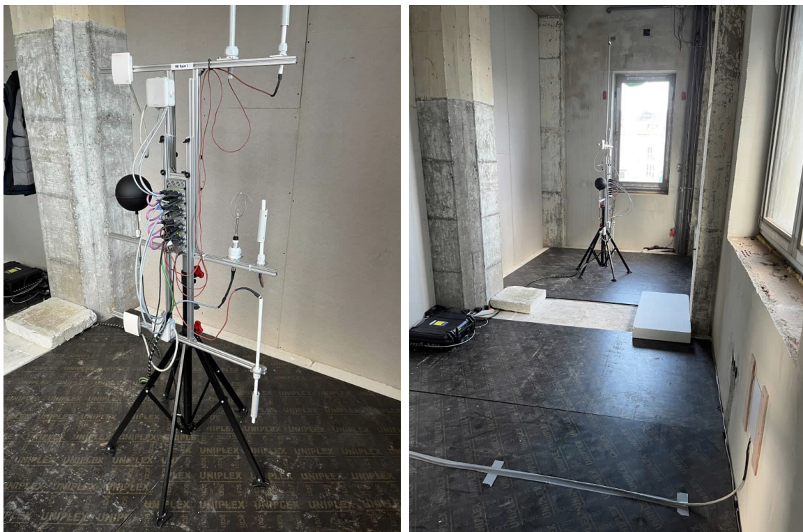
Figure 37: Realized demo room setup from the inside with comfort and heat flux measuring equipment
